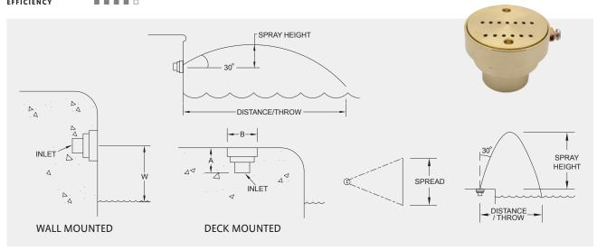
\*Contact Crystal Fountains for detailed specifications, installation and operation details.
