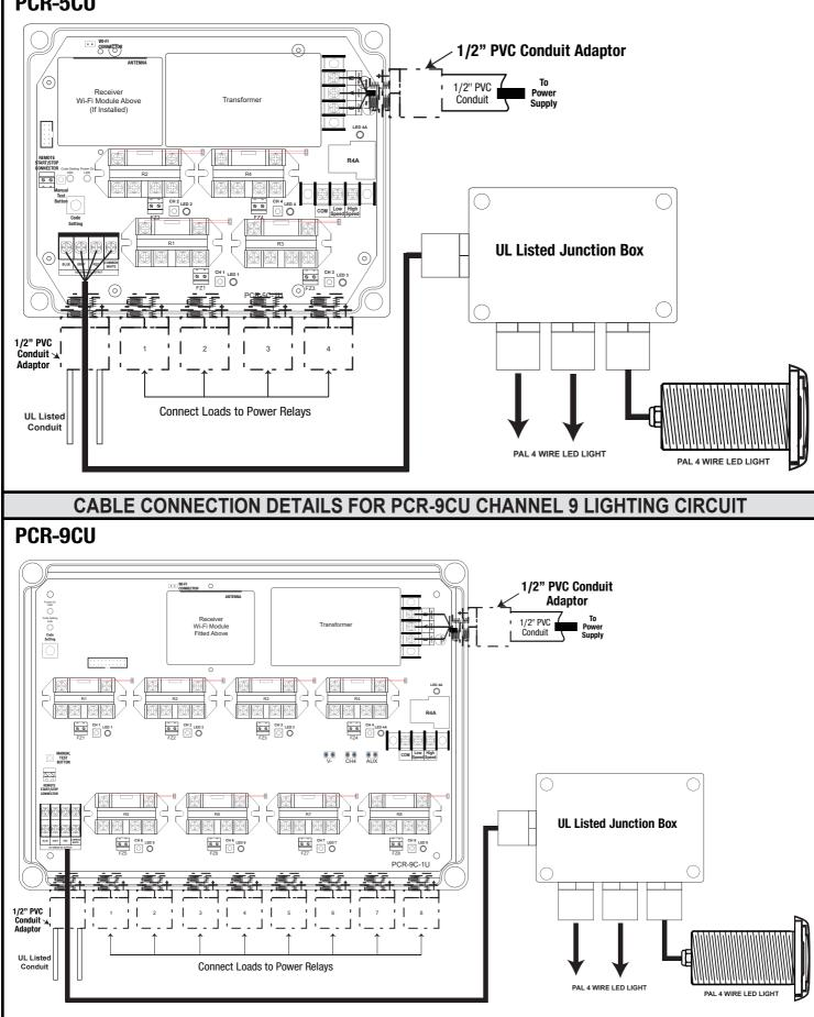
Step 1. Using the conduit entries at the bottom of the PCR-5C/9C (as shown). Connect the 4 core wire from the PAL 4 WIRE LED LIGHTS. Please ensure the 4 cores are connected to the correct terminals.
