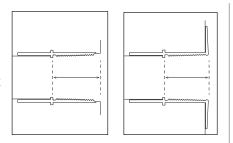
Do not install in fittings with less than 0.89" (22.6mm) of depth. If the distance is between 0.89" and 1.26" — Mod-Lite will fit. If the distance is between 0.89" and 0.94" — Remove the foam spacer If the distance is between 0.95" and 1.26" — Keep the foam spacer
