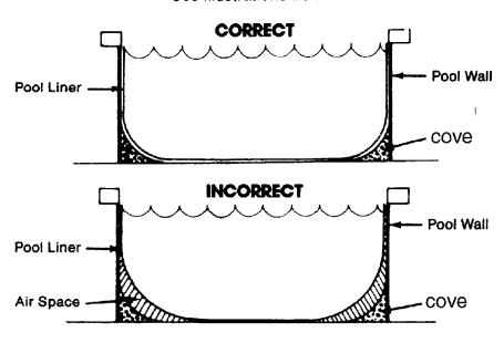
Failure to follow installation instructions will damage the pool liner and void the warranty.
