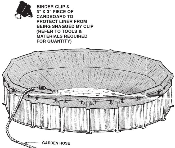
BINDER CLIP & 3" X 3" PIECE OF CARDBOARD TO PROTECT LINER FROM BEING SNAGGED BY CLIP (REFER TO TOOLS & MATERIALS REQUIRED FOR QUANTITY)
