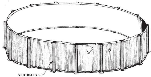
Carefully follow details shown below to assemble verticals to pool, use exploded view for your pool. Use all necessary hardware. Refer to parts list for correct screw locations. Check pool for roundness by measuring across the pool from side to side. Pool diameter should be the same from point to point.
