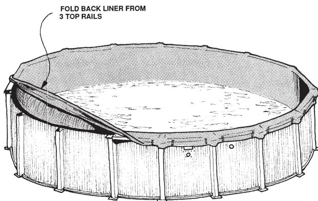
With the help of two or three people, raise and hold the liner up from any three top rail sections. Remove four top connectors, three top rails and two vertical end caps. **REMEMBER, NEVER ALLOW LINER TO FALL BACK INTO POOL.**
