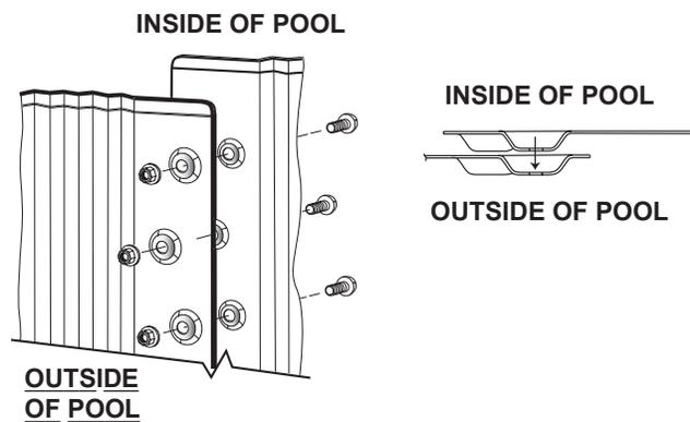
If interlocking wall ends do not meet, adjust all bottom connectors in or out uniformly as required. Do not make the total adjustment with only one or two bottom connectors. Fasten wall with screws supplied in wall carton. Screw head must be on the inside of pool. When finished, go back and retighten all screws and nuts. Remove any burrs on all screw heads. Place protective vinyl strip, included in hardware pack, over screw heads and tape in place.
