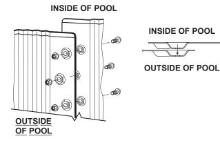
If interlocking wall ends do not meet, adjust all bottom connectors in or out uniformly as required. Do not make the total adjustment with only one or two bottom connectors. Fasten wall with screws supplied in wall carton. Screw head must be on the inside of pool. When finished, go back and retighten all screws and nuts. Remove any burrs on all screw heads. Place protective vinyl strip, included in hardware pack, over screw heads and tape in place.
