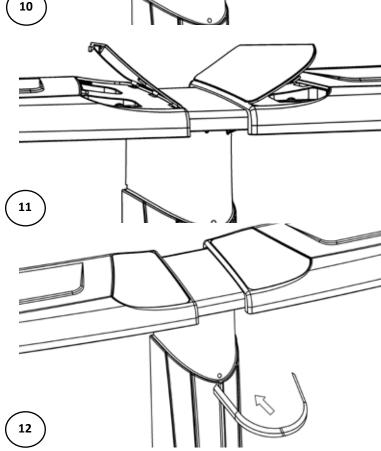
d. Install the crown at the top of the upright. Insert the central coupler into the holes and clip on the two extremities behind the upright. (Image 12)
