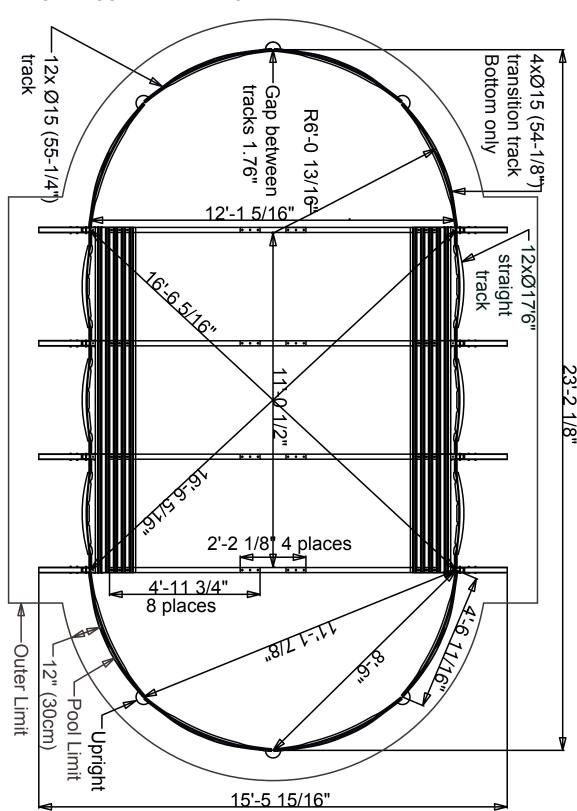
Perimeter 723" (hole to hole)- Track length measured in track slot-All dimensions are in inches
