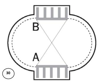
Perimeter 631" (hole to hole)- Track length meAsured in track slot-All dimensions are in inches
