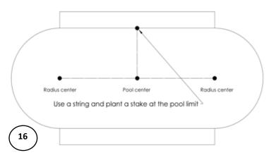
b. In order to ensure that your line is perpendicular, measure from each radius center to the top of your line. The measurement should be exactly the same on each side. If not, adjust until both are the same and you will now have a perfect perpendicular line, therfore creating a perfect 90 degree angle. (Images 17 & 18)
