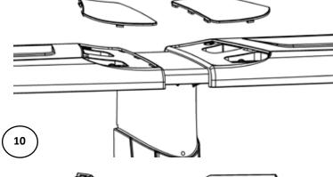
c. Start the top ledge cover installation by positioning the piece into an angle of 45 degree to insert the interior clip into the openings of the top ledge. Pivot the piece and insert the other side into the openings of the top ledge. (Image 11)
