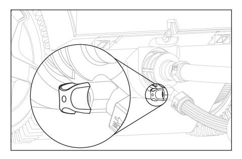
SWEEP HOSE MOVES SLOWLY OR NOTATALL: turn the adjustment knob counter-clockwise to increase sweep hose power.
