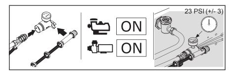
Use a flat blade screwdriver to adjust the wall quick connect knob to reach 23 PSI (+/- 3)
