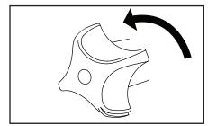
SWEEP HOSE FREQUENTLY SPRAYS OUT OF THE POOL: turn the adjusment knob clockwise to reduce sweep hose power.
