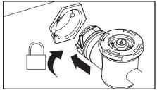
Connect pressure hose with the wall quick connect
