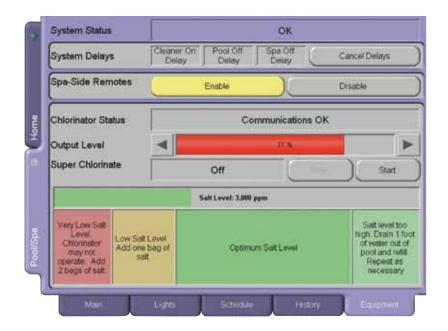
The Automatic Chlorine Generator interface enables customers to monitor their chlorinator from their controller, rather than visiting the equipment pad. Compatible with Pentair's IntelliChlor chlorine generator, as well as Goldline Controls, AutoPilot and AutoClear.
