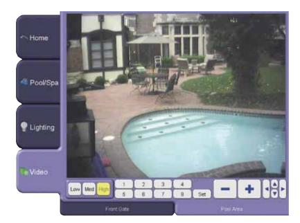
For added safety and security, owners can monitor their pool, spa or backyard with the Video screen interface. This feature supports up to four Panasonic<sup>®</sup> video cameras that send video images to every ScreenLogic interface device. These cameras support motion detection and can be set up to automatically take a picture when motion is detected and send the picture to any e-mail address.
