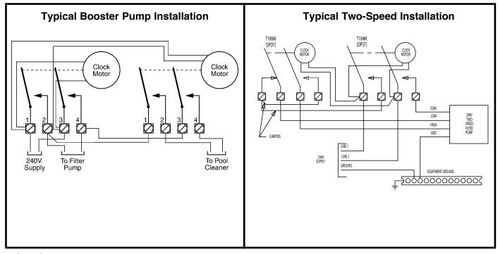
**NOTES:** 1. Grounding connections are not shown but must be provided. Refer to the National Electrical Code for details. 2. Diagrams above are only two of the many variations this Panel can accommodate.
