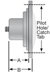
\*J&J Electronic's faceplate diameter is larger than the standard SwimQuip faceplate. Ensure there is enough even surface for fixture faceplate to fit flat against
