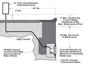
1. Feed the fixture cora unrough the conduit to the junction box. Be sure to leave at least four (4) feet of cord at base of the fixture to coil around the light to ensure ease of servicing once the pool and/or spa is filled; reference Figure 1
