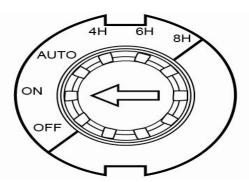
This transformer includes a photocell feature that allows light fixtures to operate either manually, on a timer, or automatically. The photocell may take up to 30 seconds to activate upon change in light levels.
