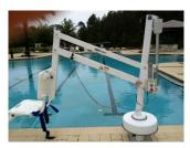
If the lift is an Extended Reach (as shown above), first check to be sure all connections are secure. Check extension cable for damaged or pinched area. Plug hand controller directly into control box. Does the hand controller work? If yes, the extension cable needs to be replaced.
