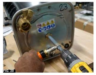
18. Cycle the Cleaning Brush shaft in and out using full strokes while rotating the shaft using the cordless drill. You may have to grip the water supply hose with one hand to keep it from rotating with the shaft.(Fig. 21).
