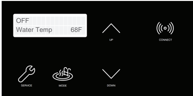
Figure 89. Wi-Fi Reset – Press and Hold CONNECT
