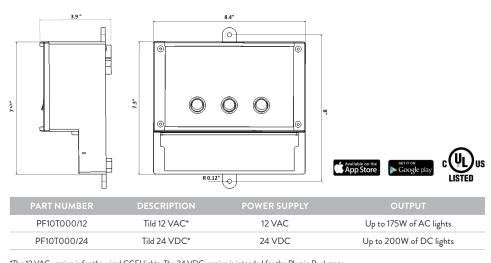
\*The 12 VAC version is for the wired CCEI lights. The 24 VDC version is intended for the Plug in Pool range.
