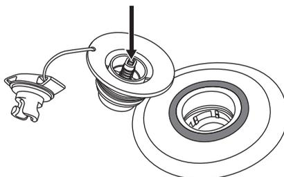
3. Check the rubber ring to make sure that it is in the correct position, secured tightly around the valve, and check that there is no debris in the way
