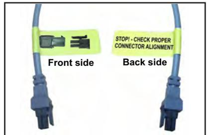
**CAUTION:** Damage may occur to the circuit board and spaside if the spaside plug is not properly aligned to the receptacle on the circuit board or if the spaside plug is connected or disconnected while the power is on.
