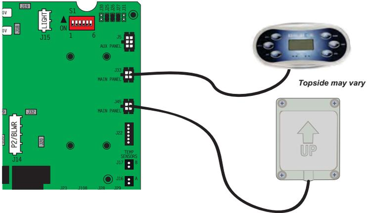
\* If no main connections are available, you may use the "Y" cable provided with the wi-fi module kit (34-51159-K)
