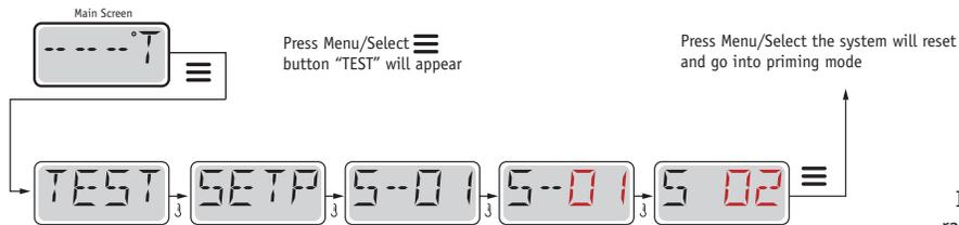
Move DIP Switch 1 to the OFF position to take the spa out of Test Mode. °F or °C will replace °T.
