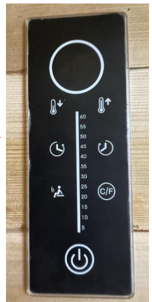
Sauna Control Panel has no Illumination
