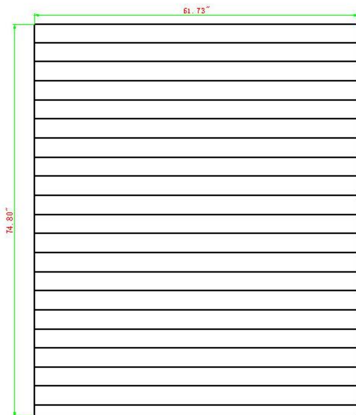
Rear wall panel
