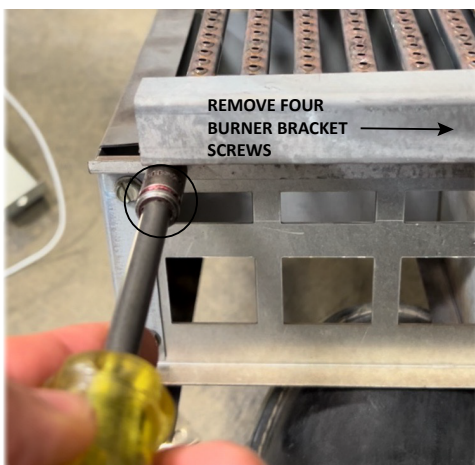
Figure 2. Remove Four Burner Bracket Screws
