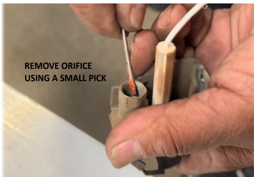
Figure 12. Remove Orifice from Pilot Cavity
