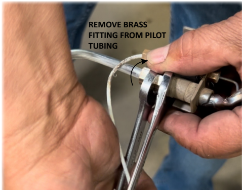
Figure 11. Remove Brass Fitting
