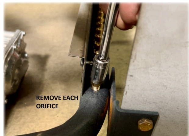
Figure 5. Remove Individual Burner Orifices
