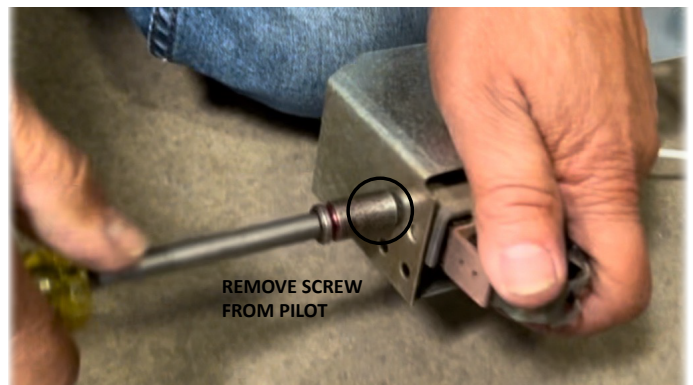
Figure 10. Pilot Assembly Removal from Bracket
