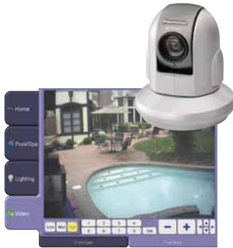
**Video Camera Support:** capable of supporting up to four video cameras and sending the video image to any ScreenLogic interface device. Requires Video and Lighting Protocol Adapter; in addition to one of the four ScreenLogic kits. (P/N 520854Z)
