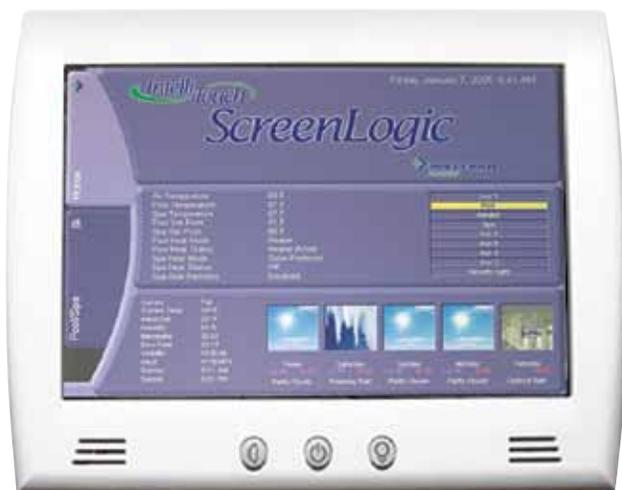
**iTC35 Kit (P/N 520502):** includes In-Wall Color Touch Screen with Ethernet (RJ45) connection and the Protocol Interface Adapter and wireless router. The touch screen device is custom-configured for IntelliTouch systems.
