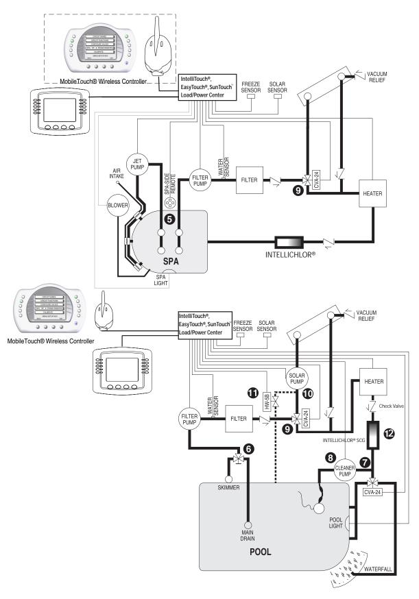
Recommended Hydraulic Schematic for Single Body System
