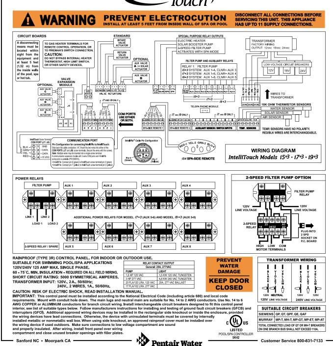
System Wiring Diagram (Load Center)
