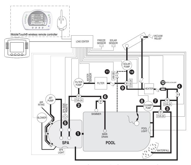
Recommended Hydraulic Schematic for Shared Equipment System
