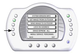
6. Press the button next to **LOCK ON ADDRESS** to assign a unique frequency for the MobileTouch controller to avoid inference from other wireless devices within range of the MobileTouch transceiver.
