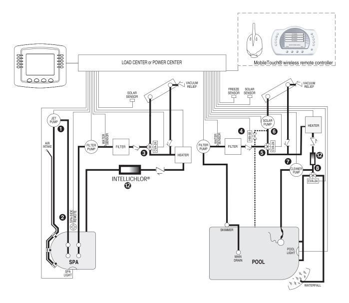
Recommended Hydraulic Schematic for Dual Equipment System
