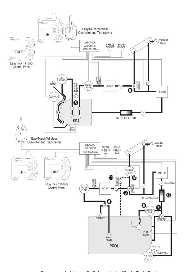
Recommended Hydraulic Schematic for Single Body System
