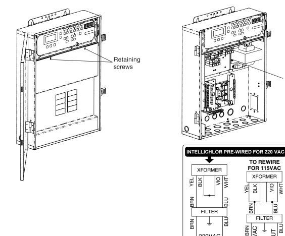
IntelliChlor transformer and filter wiring diagram
