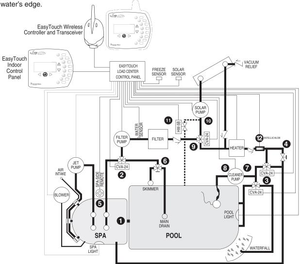
Recommended Hydraulic Schematic for Shared Equipment System
