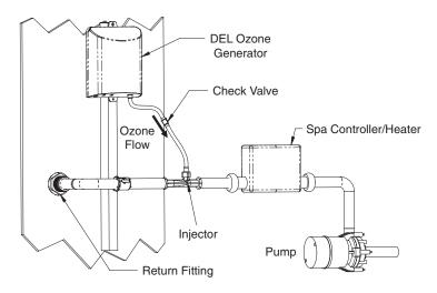
Figure 1: Typical Injection System
