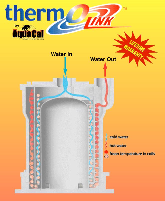
The only patented titanium system that uses counter flow water management to maximize temperature differential and heat transfer.
