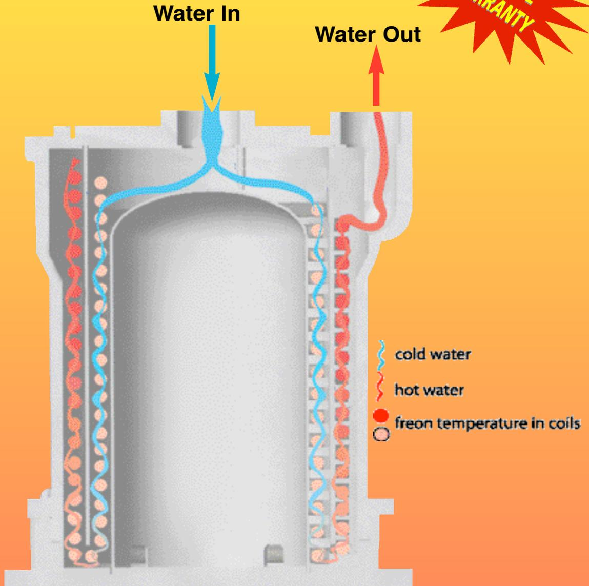
The only patented titanium system that uses counter flow water management to maximize temperature differential and heat transfer.
