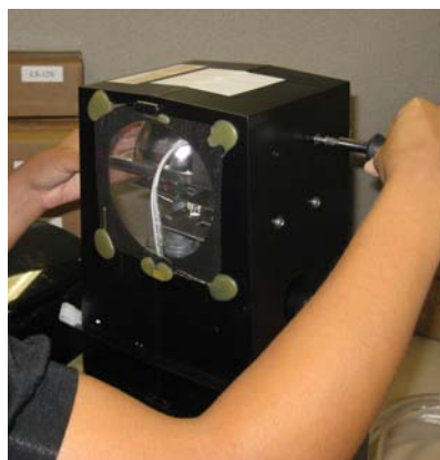
... unscrew top two Phillips head screws as shown
