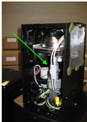
Locate the indicated 2-wire lamp connector plug
