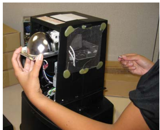
Carefully remove the old Y20-6000 from the illuminator chassis
