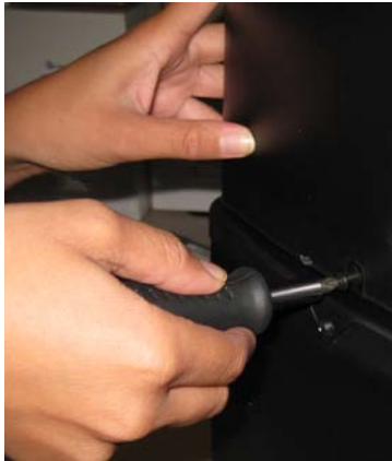
Remove upper Phillips head screws located on the front and back of 6004 cover
