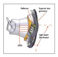
Drawing shows unique lens and reflector designs which combine to provide superior light beam distribution.
