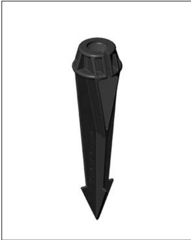
This 8" spike is the standard for all FX uplites and small pathlites. Constructed from UV resistant ABS it incorporates a composite thread insert featuring a slot cut out of the threads for your wires. No fumbling with the wires when trying to attach the spike!
