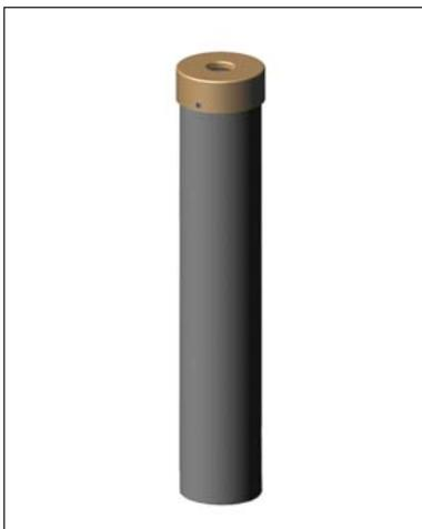
For commercial projects or where a clean finish is needed for the cable connection specify the Post Mount®. Milled from solid brass or aluminum alloy and powdercoated to match any standard FX finish. Includes 12" PVC pipe mount. Sturdier than the Super J-Box® when cast into a concrete footer. 2.50" x 12.50"
