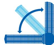
Unique folding ball joint design allows lateral assembly to be easily accessed for simple servicing.
