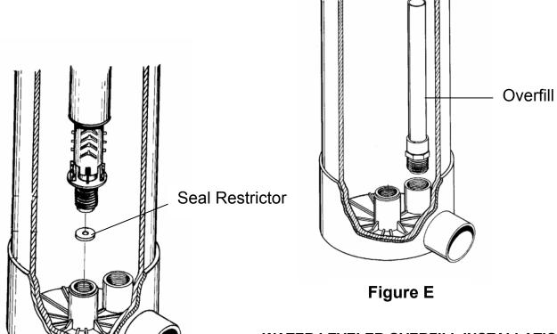
WATER LEVELER OVERFILL INSTALLATION
