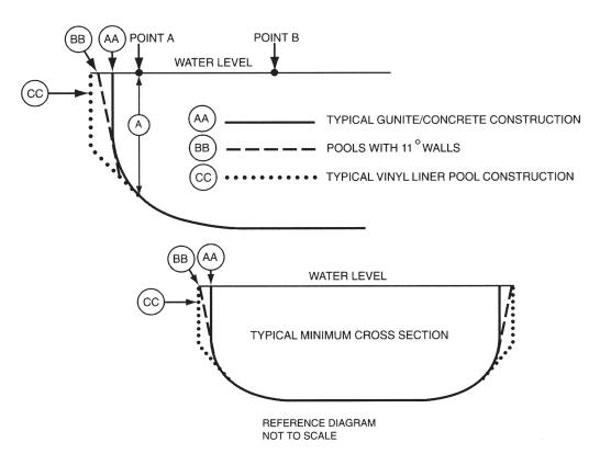
Figure 2 – Typical pool design configurations
