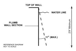
Figure 1 – Maximum allowable wall slope
