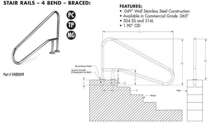
**NOTE:** Escutcheons sold separately w/SS products; included with powder coated and thermo plastic coated ladders and rails. *All measurements on center.* Anchors are not included and recommended.
