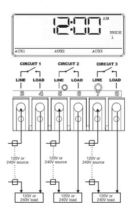
Mode 2 – (Pump High, Pump Low, Aux3) Circuit one and two are dedicated single pole outputs for a two-speed pump load. Circuits one and two will never be ON at the same time, consistent with a two-speed pump application. Circuit three is single pole circuit for a generic load, and independent of circuits one and two.
