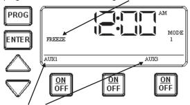
Aux #1 & #3 will blink indicating the control has activated these two circuits due to a freeze condition. To override the circuits during a freeze condition, simply press and release each of the corresponding ON/OFF keys. This will override the freeze control and turn the devices OFF. The override will only last for one hour, so if the freeze condition still exists after one hour, circuits #1 & #3 will come back on.
