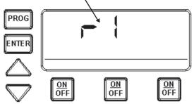
3. Release the **ENTER** key after viewing the revision level. The revision level should disappear and return back to the time of day.
