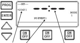
Circuit #1's first event has not been defined. You have the ability to program up to three separate events per load or circuit. An event is defined as a complete On and Off cycle.
