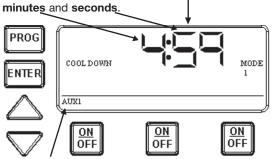
The **AUX1** indicator is blinking indicating the cool down feature is activated for circuit #1. When the count down display reaches **zero**, the actuated circuits - (#1 or #2) depending on mode (2 or 4), will open and the display will change back to the time of day.
