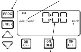
The default cool down time is zero. Use the arrow keys to modify the cool down time. The range is zero to fifteen minutes. Use the Enter key or Program key to either save and exit, or save and advance to the next programming feature.
