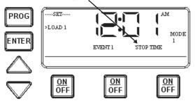
4. Use the Up and Down arrows keys to define the stop time for circuit #1's 1st event. Press and release the Enter key when complete. The program will now advance to the **second event** for circuit #1.
