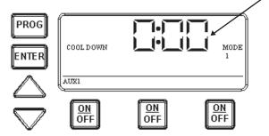
You can override the cool down feature by simply pressing and releasing the ON/OFF key associated with circuit #1. This will end the cool down cycle, and immediately turn off circuit #1.
