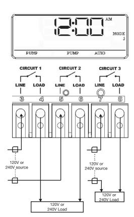
**Mode 4** – (Pump High, Pump Low, Cleaner Pump) Circuit one and two are dedicated single pole outputs for a two-speed pump load. Circuits one and two will never be ON at the same time, consistent with a two-speed pump application. Circuit three is also a dedicated single pole output for a pressure side cleaner pump. Circuit three will never come on unless circuit one is on for at least one minute, consistent with a pressure side cleaner pump.
