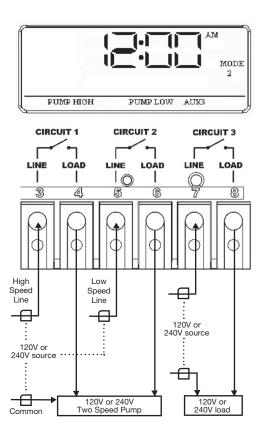
**Mode 3** – (Pump, Aux2, Cleaner Pump) Circuit one and three are dedicated single pole outputs for a single speed pump working with a pressure side cleaner pump. Circuit three will never come on unless circuit one is on for at least one minute, consistent with a pressure side cleaner pump. Circuit two is a single pole circuit for a generic load, independent of circuits one and three.
