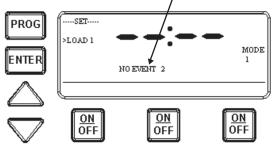
The display indicates, no 2nd event for circuit #1 has been defined. Follow the previous tasks 2 thru 4 to set a second event for circuit #1.
