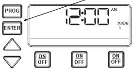
2. After 5 seconds, the display should change to the revision level. The r1 stands for revision one, r2 for revision two and so on.
