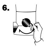
Insert the non-lipped end of snap ring into the groove opening beginning at the 5 o'clock position and push it up so that it threads itself around the control dial.
