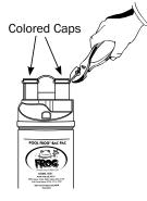
Remove colored caps by grabbing on to the lip of one cap with a pliers and pulling up until cap releases. Repeat the process for the other cap.
