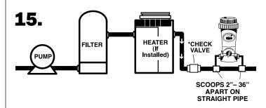
To prevent damage to heaters or filters, see your dealer about installing a corrosion resistant check valve which will reduce the back flow of chlorine gas when the Cycler is turned off.
