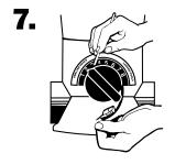
Using a small screwdriver or pointed tool to help guide it, make sure the snap ring stays in the groove as it is inserted.
