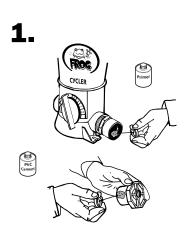
Following Primer directions, brush Primer on reducer bushings and inside of male adapters. Repeat this process with PVC cement following manufacturer's directions on that product.
