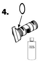
Carefully replace the rubber O-ring without stretching it. Apply silicone lubricant, that came with your Pool FROG Cycler, on O-ring.
