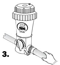
Insert PVC pipe into adapters with a twisting action. Hold in place 5 to 10 seconds to bond.
