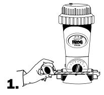
Measure the distance between the outside adapters and cut out a section of pipe 3" less than that dimension.
