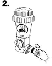
Insert reducer bushing into male adapter on both sides with a twisting action. Hold in place 5 to 10 seconds to bond.
