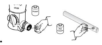
Following Primer directions, brush Primer on the inside of the adapters and to ends of pipe. Repeat this process with PVC cement following manufacturer's directions on that product.
