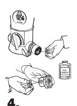
Following PVC cement directions, brush PVC cement on reducer bushings and inside of male adapters.
