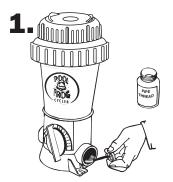
Following pipe thread sealant directions, brush sealant on to POOL FROG® Cycler threads in both ports.
