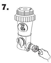
Screw elbow into reducer bushings on both sides.
