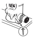
Use Phillips pan head screws through the mounting holes at the POOL FROG® Cycler base to secure the POOL FROG® Cycler into a treated wood base.
