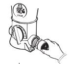
Screw a male adapter into each port of POOL FROG® Cycler and hand tighten.
