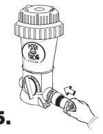
Insert reducer bushing into male adapter on both sides. Hold in place 5 to 10 seconds to bond.
