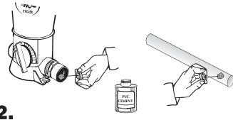
Following PVC cement directions brush PVC cement on the inside of the male adapters and to ends of the pipe.
