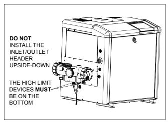
Figure 12. Water Connections Reversed
