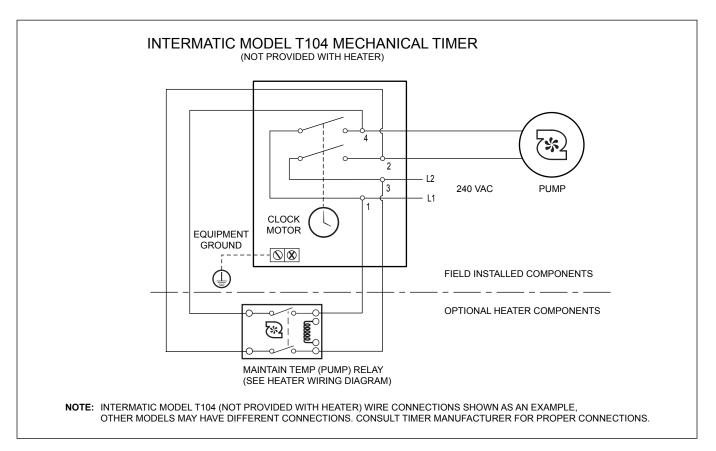
Figure 24. Example of Maintain Temp Wiring to the Time Clock
