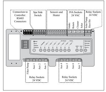
Figure 27. PCB Board with Firmware REV MMM or
