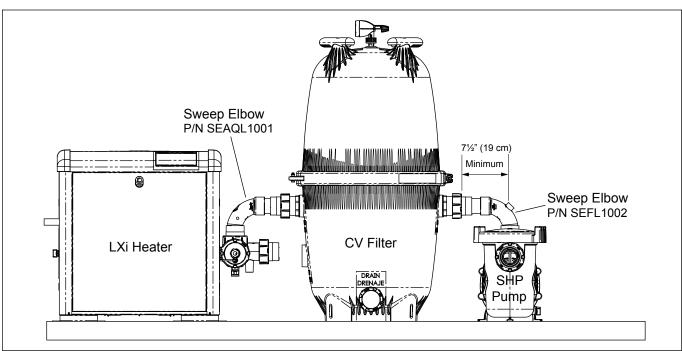
Figure 16. LXi Heater Sweep Elbow Installation
