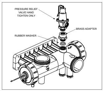
Figure 19. Pressure Relief Valve Installation
