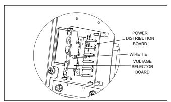
Figure 23. Power Distribution Board With Voltage Selector Board Installed for 240 VAC
