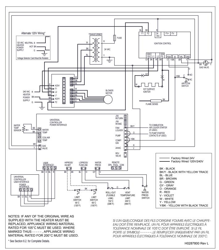
Figure 20. LXi Connections/Schematic Wiring Diagram
