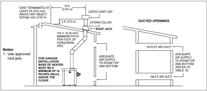
Figure 7. Indoor Installation Venting (USA), or Outdoor Shelter (Canada)
