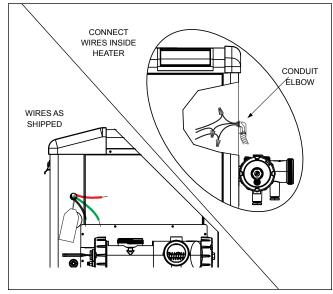
Figure 21. Field Wiring Connections
