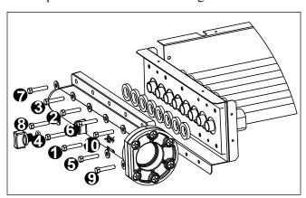
Figure 14. Header Bolt Tightening Sequence
