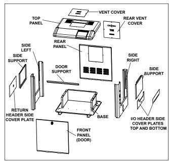
Figure 13. LXi Panel Identification
