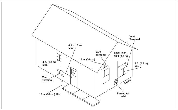
Figure 8. Side Wall Vent Terminals
