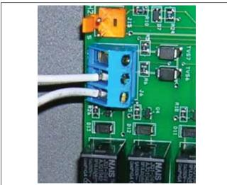
AquaLink® RS or Remote TSTAT Connection Figure 26. (2-Wire Connection)
