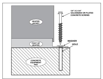
**Anchor Heater To Equipment Pad** Figure 4.
