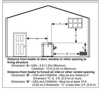
Figure 3. **Outdoor Heater Installation**
