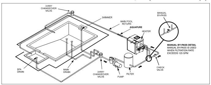
Figure 10. Typical Piping Installation
