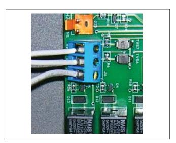
Figure 25. Remote Pool-Off-Spa Connection (3-Wire Connection)
