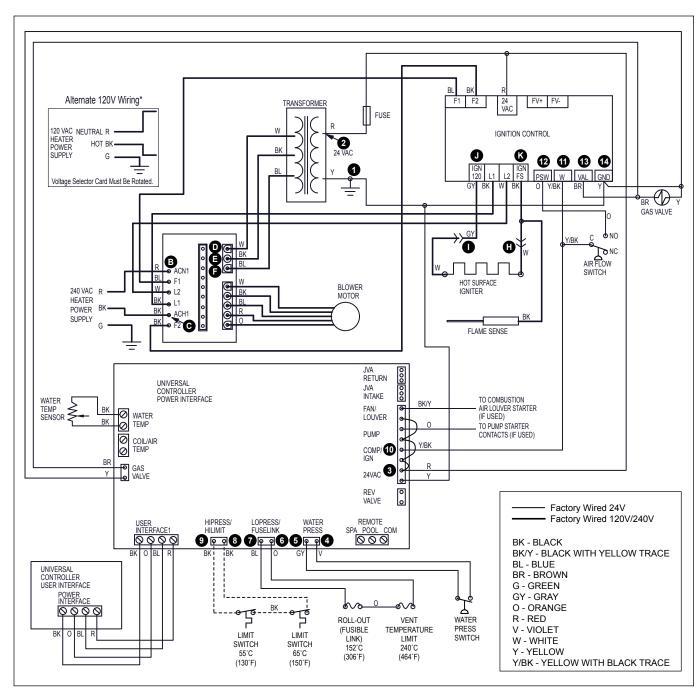
Figure 39. Test Point Identification Diagram
