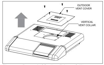
Figure 5. Removal of Outdoor Exhaust Grill
