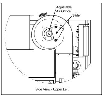
Figure 37. Adjustable Air Orifice Location
