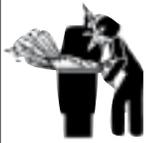
Follow all filter manufacturer's instructions. **NEVER** attempt to assemble, disassemble or adjust the filter when there is pressurized air in the system. Starting the pump while there is any pressurized air in the system can cause the filter lid to be blown off, which can cause death, serious personal injury or property damage.
