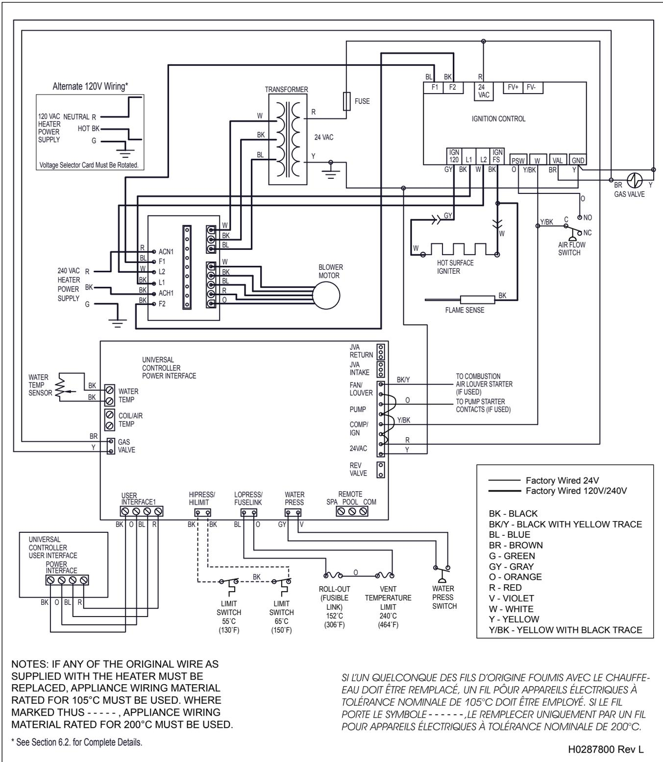
Figure 20. LXi Connections/Schematic Wiring Diagram
