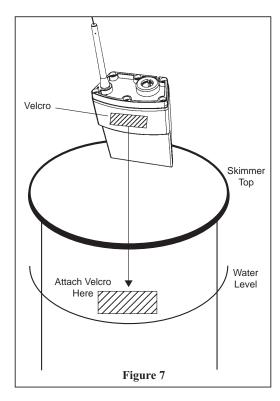
Transmitter can be re-set at any time by simply placing the Transmitter higher or lower on the velcro attached to the Skimmer. Additional velcro can be attached to the Skimmer if necessary. The Transmitter antennae is flexible and will bend over when the Skimmer lid is replaced. Do not change the length of the antennae.
