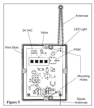
or off signal (*See Section 2.3*) the LED will go on for 2-3 seconds indicating that the transmission has been received. This is a way to check that the unit is working.
