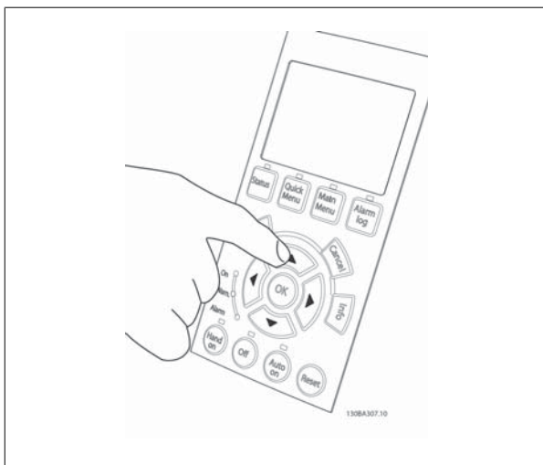
Illustration 5.51: Step 6: The speed of the motor can be seen in the LCP. It can be adjusted by pushing the up ▲ and down ▼ arrow buttons.
