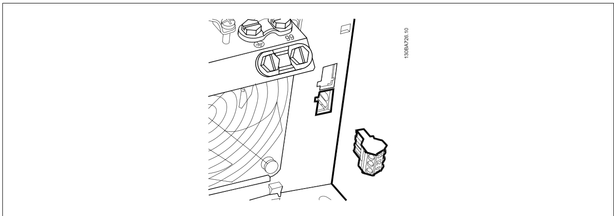
Illustration 5.38: Terminals for relay connections for B3. Only one knock-out is fitted from the factory.
