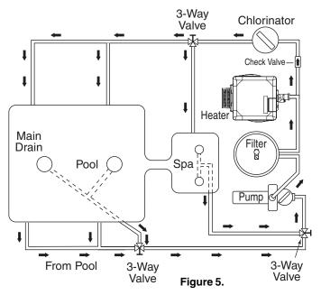
Install the chemical feeder downstream of the heater. Install a chemical resistant one-way check valve between the heater and the chemical feeder to prevent back-siphoning through the heater when the pump is off.
