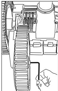
Once off, fold the tire off the Wheel Hub (step 3 above). To replace stretch the tire over the
