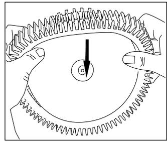
**4** **BACK TIRES** remove the Wheel Hubs with a 5/32" or 4mm allen wrench turning the wrench counterclockwise.
