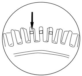
**3** Place the cleaner on a work surface. **TO REMOVE THE POOL-CLEANER™ FRONT TIRES**, use only your hands (other objects may damage the POOLCLEANER™) simply fold the tire off from top to bottom.
