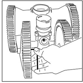
**Note:** The front tires **ALWAYS** have **HUMPS** (raised treads) The back tires **DO NOT** have humps!
