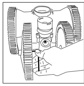
**6** Rotate the right front tire forward to ensure that it moves smoothly. If not you fastened the wheel hub incorrectly.
