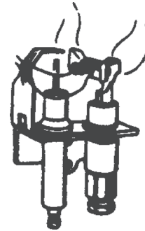
Fig. 33: Pilot Burner Flame
