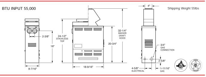
An electronic heater using propane gas is "EP"; an electronic heater using natural gas is "EN". A Millivolt heater using propane gas is "MP"; a Millivolt heater using natural gas is "MN". Prefix "B" is for brass headers. Suffix "C" is for copper tubing.
