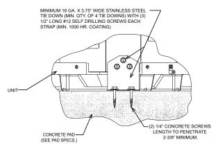
HIGH WIND LOAD RESTRAINT DETAIL 1
