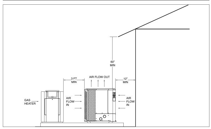
Fig. 1: Installation Clearances
