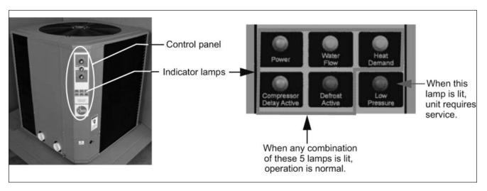
Fig. 3: Indicator Lamps — Analog Models
