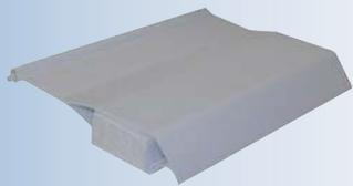
The unique patented hydrodynamic weir in the skimmer creates a lifting action on the skimmer plate, much like an airplane wing. This uplift speeds up the surface flow and eliminates ineffective deep currents. The Hydro-Skimmer skims a thinner layer of surface water at a higher velocity, resulting in 300% to 500% more surface skimming and it does it at flow rates as low as 10 gallons per minute.
