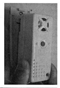
mounting bracket. You will feel a click when the unit is properly installed.
