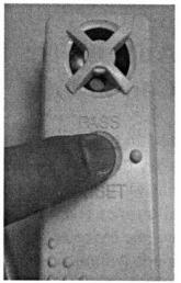
To reset the alarm, first close the door and then press the PASS/RESET button. The alarm is now back to stand by mode.
