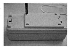
Now the unit is ON and in working mode. To check if battery is installed properly, press the battery check button located at the lower right corner. The unit will beep when you press this button. If no beep sound is heard, check the battery installation again,
