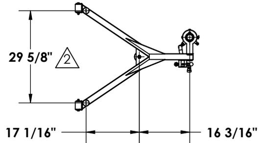
△2 Note: Clear deck space shall be provided parallel to the water 36" wide x 48" minimum from a line located 2" behind the rear edge of the seat. (15.8.5.3 ADA Guidelines)
